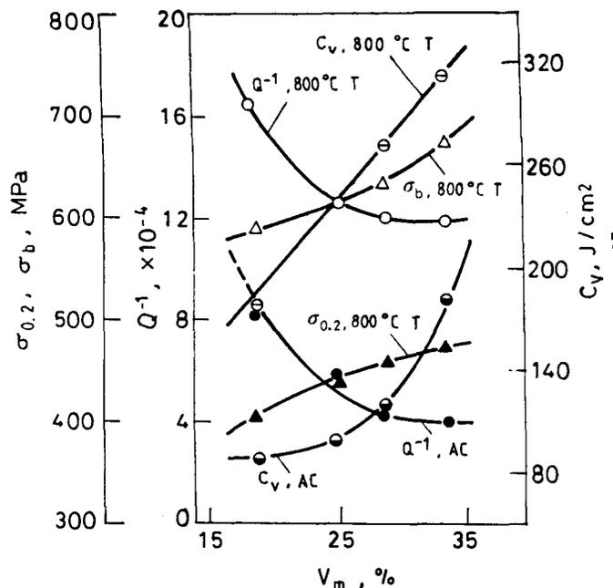
Fig. 1 Effect of martensite volume fraction on mechanical properties and damping capacity.
